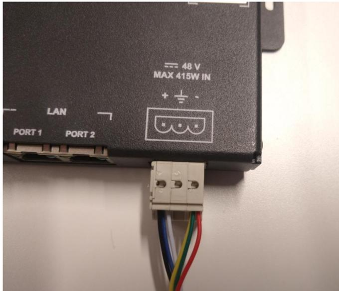
**Note: With this solution you only have 200W power available. So you can only connect devices consuming up to 200watt in total!**
