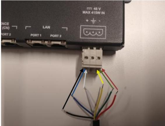
To insert the wires in the WAGO connector you will need to use a flat screwdriver. You first need to insert the screwdriver in the connector to open the wire-clamp. Then you may insert the wires in the WAGO. If the wires are properly inserted in the connector you may release the screwdriver. This ensures that the wires are securely seated in the connector. **Check if the wires are securely seated in the connector before continuing!**
